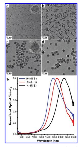
**Figure 1.** Transmission electron microscopy images of ITO NCs of varying size (nm): (a)  $4.1 \pm 0.6$ , (b)  $7.4 \pm 1.4$ , (c)  $10.2 \pm 1.7$ , and (d)  $12.1 \pm 1.5$ . (e) Extinction spectra of NCs with varying tin content (%) in solvent dispersions.
