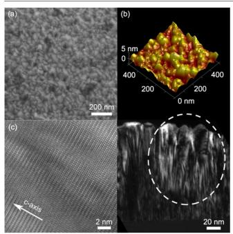
**Figure 1.** (*a*) SEM, (*b*) AFM, (*c*) cross sectional TEM and (*d*) dark field  $(0\,0\,2)$  TEM of AZO grown by dc arc. Images come from three different, typical samples with the TEM images taken on the same sample. A grain is circled in (*d*) with the dotted line.
