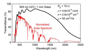
**Figure 2.** Transmittance of AZO/glass grown by the compact dc arc system (not corrected for the substrate). The AM1.5 solar spectrum is shown in relative units for comparison and the electrical properties of this film are in the upper-right corner.
